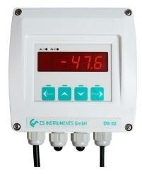
With the digital process meter DS 52 in a shapely wall housing the annoying search and the mounting into a suitable plastic housing is no longer necessary. DS 52 disposes of 2 potential-free alarm contacts (switch-over contacts) which can be charged with maximum 230 VAC, 3 A. The alarm limits can be adjusted via the keys.
